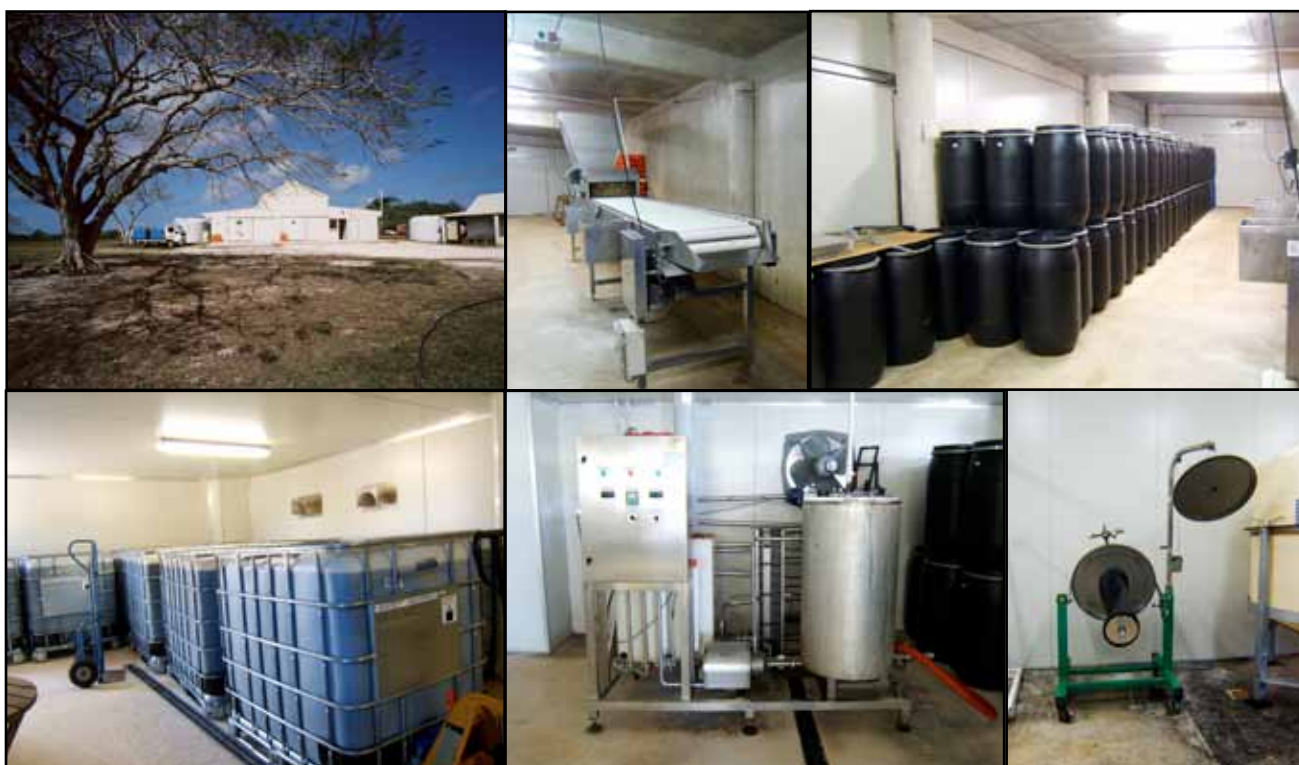
Clockwise from top: Reef's noni processing plant on Vaiea farm; Fruit is washed and graded; then matured in airtight barrels; Hydra-presses designed for the wine industry are used to gently squeeze the juice out of the fruit. The equipment works perfectly well for Noni; When approximately 10,000 litres of juice is produced, it is pasteurised; Juice is then packed into 1000 litre IBCs for export.
